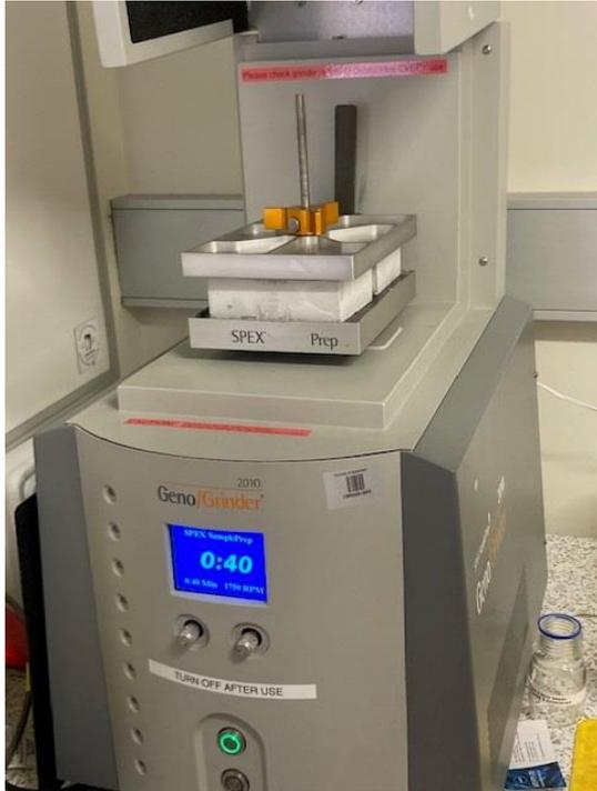
Figure 2: Make sure the orange screw is fastened tightly (if not, it will make a big noise. Immediately stop machine if this noise occurs)
