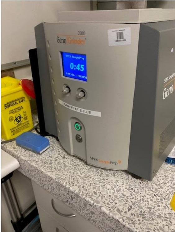
Figure 3: Press start to grind for allotted time at max speed. The green button is the start button.
