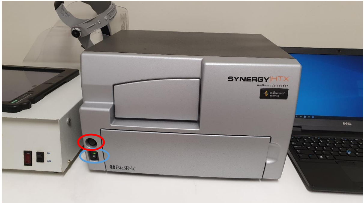
Figure 4: Tray (red circle) and OFF (blue circle) button on the plate reader
